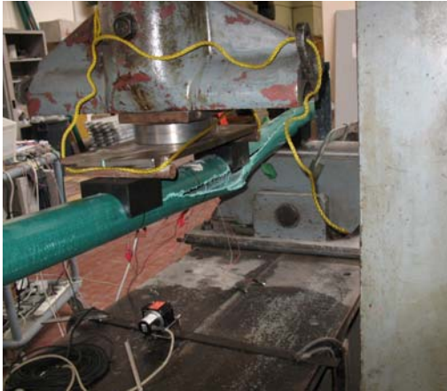
Figure 10: Shear failure in test 5
