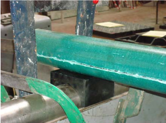
Figure 8: Shear failure in test 4
