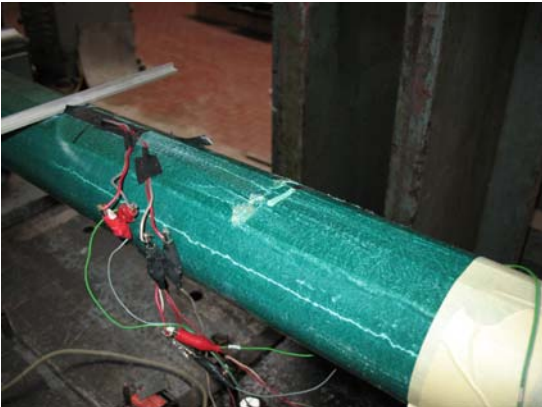
Figure 6: Local punching failure in test 1
