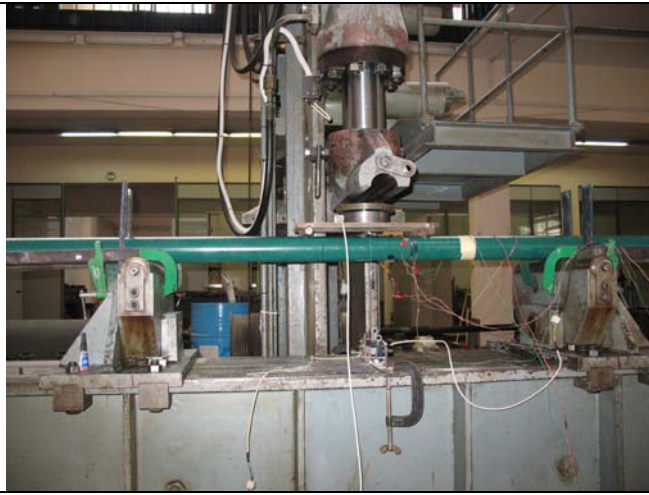
Figure 4b: Pipe specimen during test
